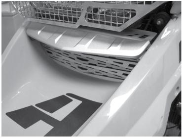
Replace the side covers and replace the (3) fasteners per side. Do not overtighten these, they only need to be firmly secured.
