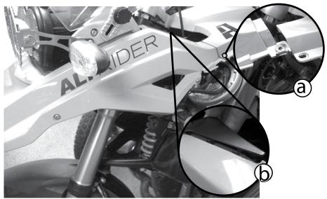
Once lined up properly, (a) be careful to make certain the fastener tab fits *under* the tank cover. Once the beak is in place, (b) don't forget to snap the plastic cover back in place.
