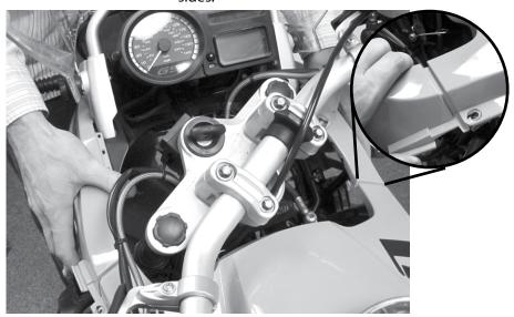
When removing the beak, be sure to use two hands, one on each side. This can be tricky, due to the adhesive BMW uses to stick the plastic to the subframe pull apart gently, but do not yank on the beak as this can cause damage.
