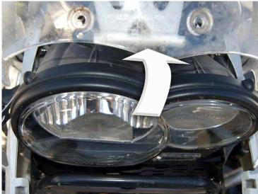
Now push the headlamp up and back toward the dash. No need to shove it, just firmly push it out of the way, slowly to make sure you don't damage anything. With the lamp moved out of the way you can install the guard as normal.
