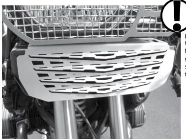
Place the oil cooler guard on the oil cooler, use the edge of the oil cooler guard to align with the oil cooler mount tabs.
