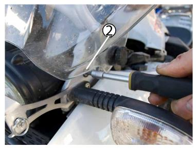
② Using a T30 tool, remove the left and right torx fasteners that hold the headlamp in place. The headlamp will now be floating in position.
